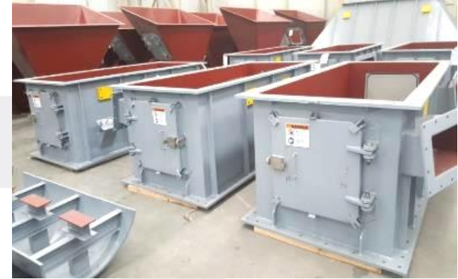
Bottom Ash Chute
