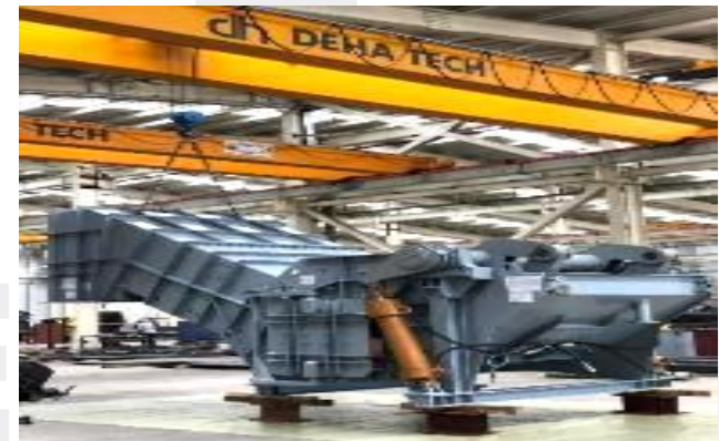
Bottom Ash Extractor
